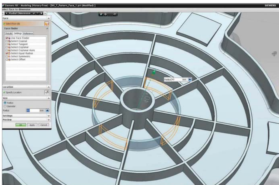
Figure 3: Sometimes you want to stagger ribs for structural strength. Synchronous technology allows you to do that with a simple cut and paste—and a change in radius.
